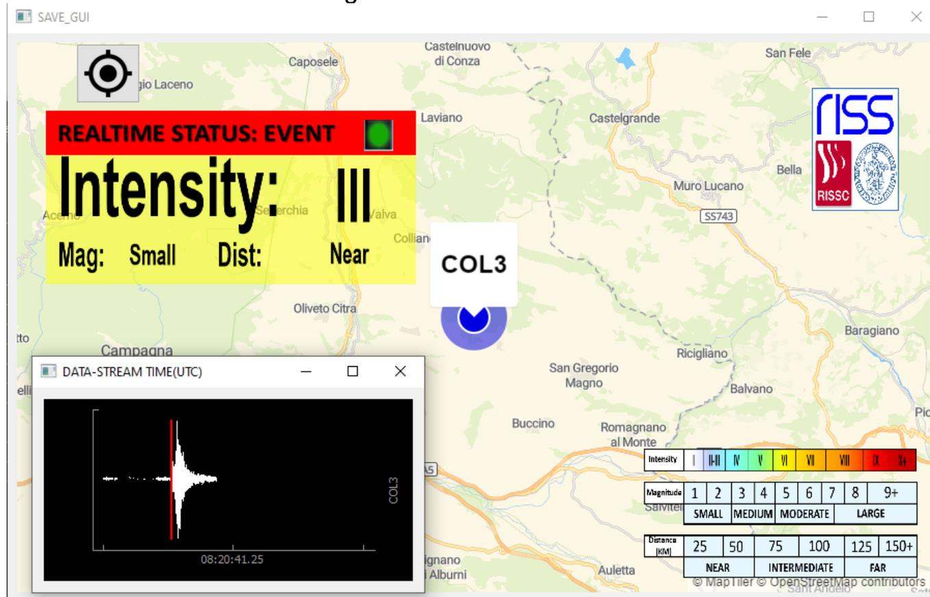
The system was able to compute both the Pd amplitude and the Tauc parameter, and was able to provide estimates of magnitude, distance and intensity ranges.
