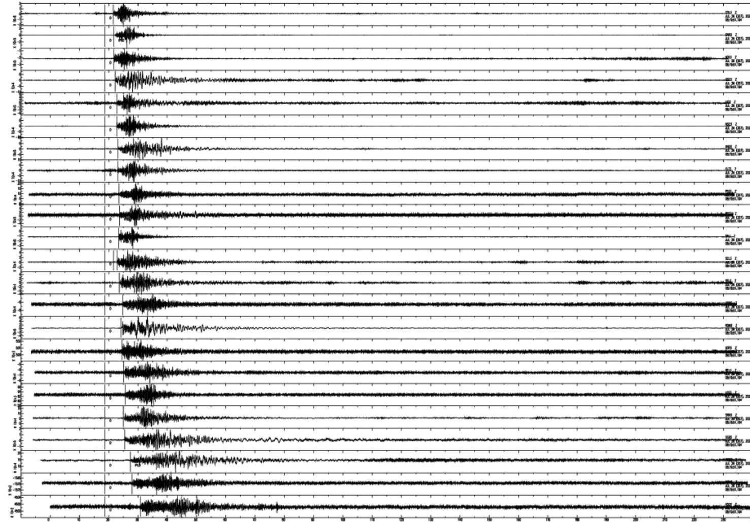
Example of **seismic waveforms (vertical component)** recorded at the stations of ISNet, for the ML 3.5 event (26/07/2023 08:20:09 UTC) in the epicentral distance range **11- 94 km.**
