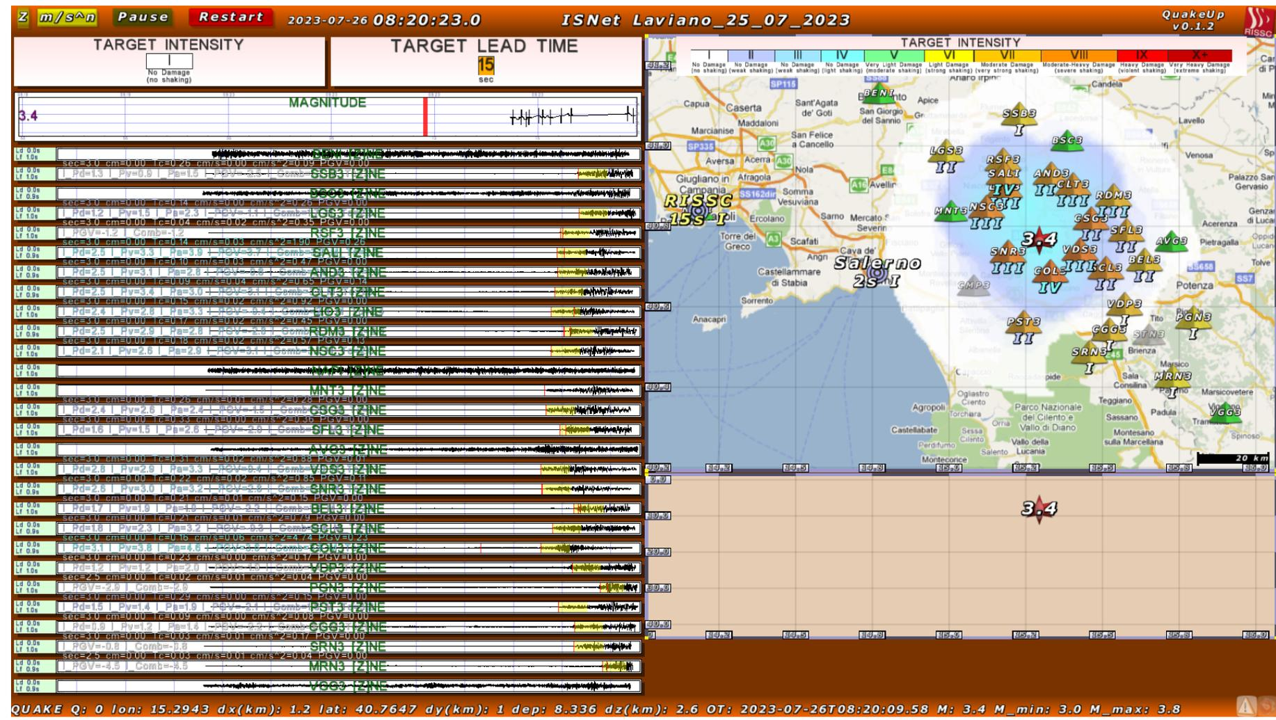
About 6 sec after the Origin time of the earthquake the system is able to predict and map the extent of the Potential Damage Zone (here represented by the IMM 3-4) using the information from early P-wave amplitudes combined with predictions from the GMPE through the real-time earthquake location and magnitude. The predicted PDZ shows a primary elongation toward NW, which is an indication for dominant rupture directivity to N-NW.
