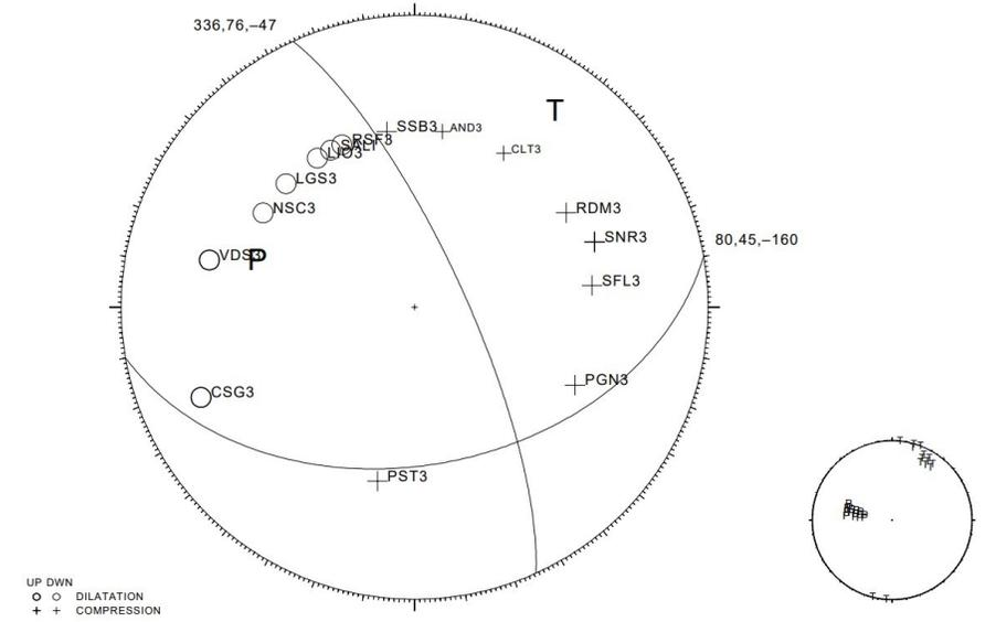
Focal mechanism solution shows a normal fault mechanism with a strike-slip component. Inversions performed using only polarities (a) and P and S amplitudes together with polarities (b-d) provide slightly different focal planes. The Kagan Angle between the two solutions is equal to  $30^\circ$ .
